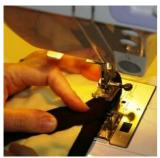
Pull the entire strip of elastic over to lay flat on top of the fleece.
